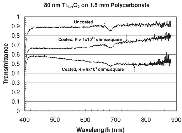
Figure 5: Optical transmittance of titanium-rich  $\text{TiO}_2$  coatings on polycarbonate.
