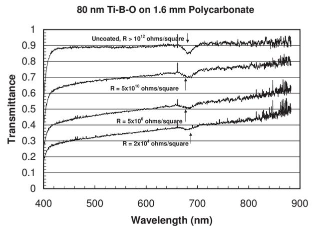
Figure 4: Optical transmittance of Ti-B-O coatings on polycarbonate.
