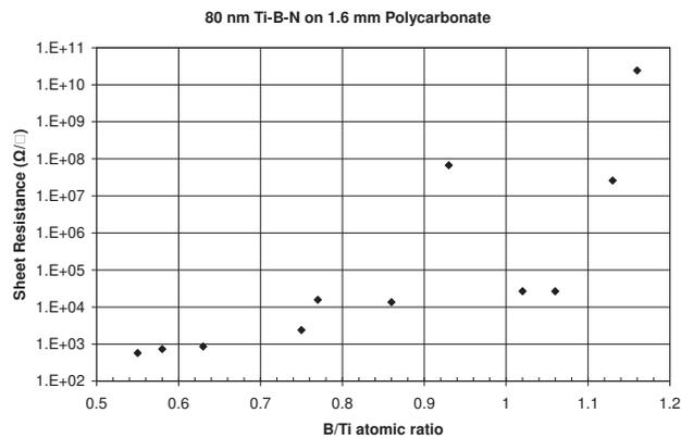
Figure 1: Sheet resistance of Ti-B-N films vs B/Ti atomic ratio (also  $\sim$  the N/Ti ratio).
