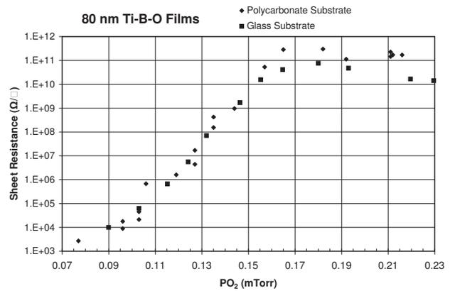
Figure 2: Sheet resistance of Ti-B-O films vs partial pressure of oxygen during deposition.
