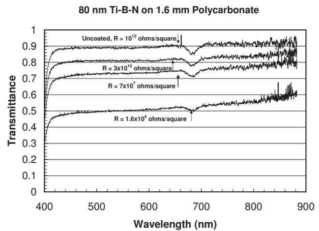
Figure 3: Optical transmittance of Ti-B-N coatings on polycarbonate. Sheet resistance ( $R$ ) of each film is shown.
